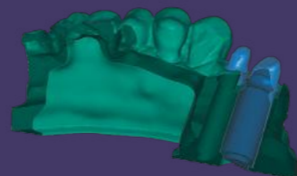
Hollow models allow extremely cost-efficient printing
